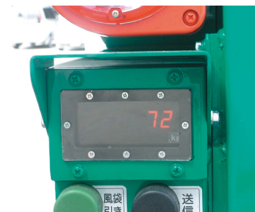
Scale Packer use to weigh the amount of waste collected
